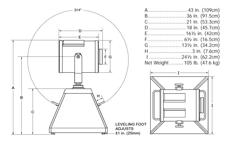
Power Requirement: 110-120 V.AC, 15 Ampere Single Phase (220-240 volt model available) Bulb: Single-Ended 1200 Watt Metal Halide (Philips MSR/MSD 1200/2 or equivalent)
